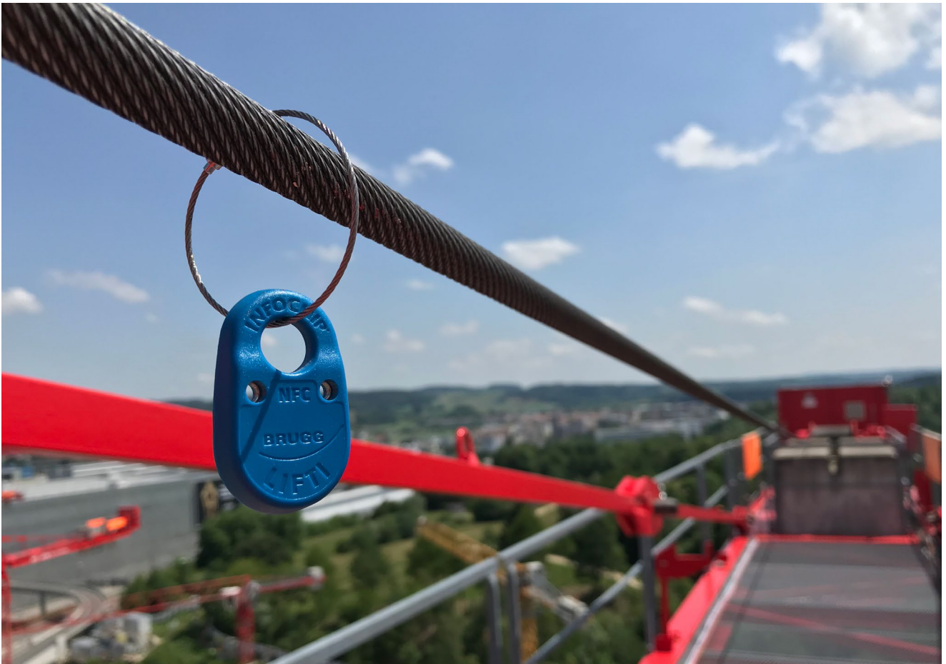
A PVS NFC tag attached to a steel rope on a construction site (BRUGG Lifting, 2018)
